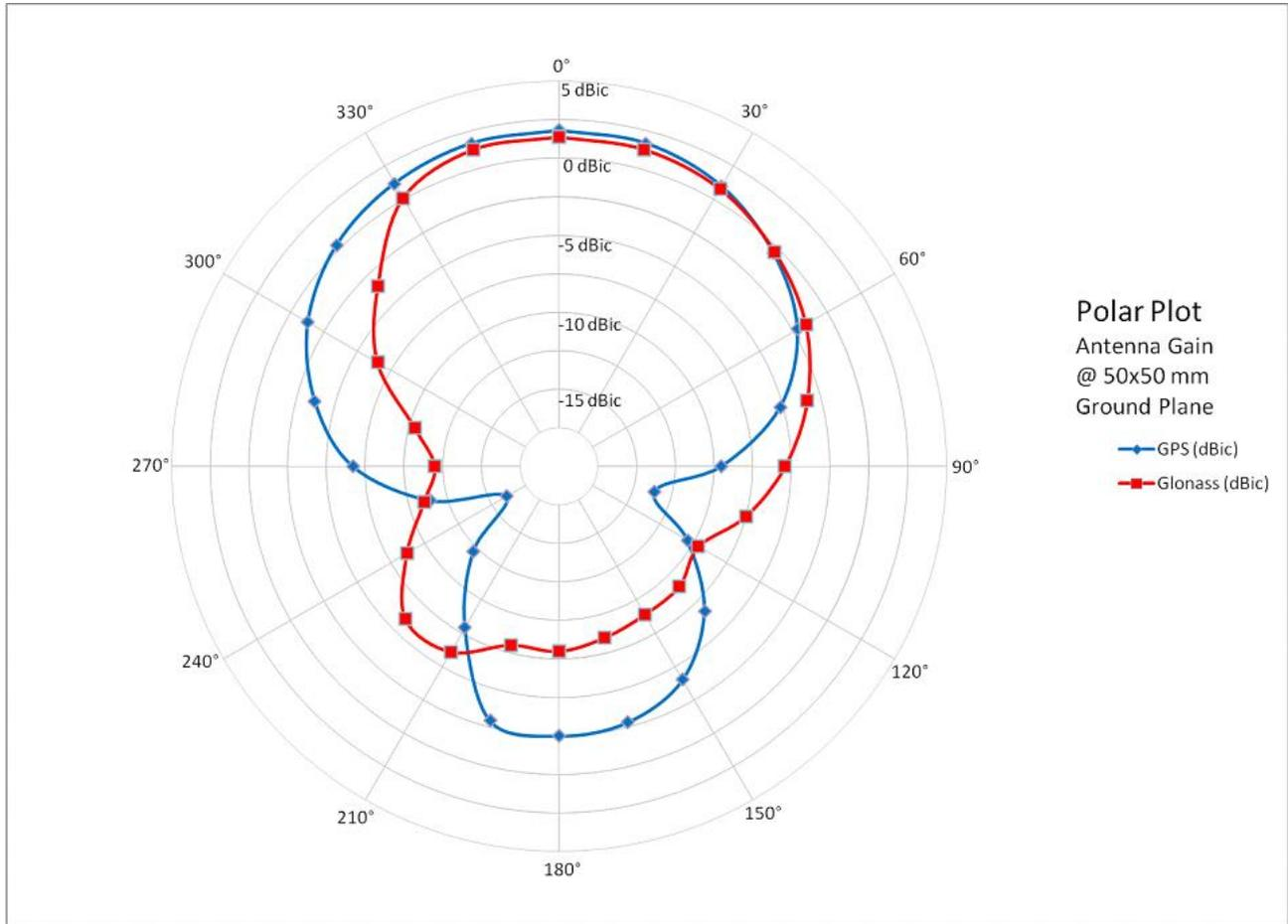
**Figure 7: 1.575 GHz typical free space radiation patterns**
