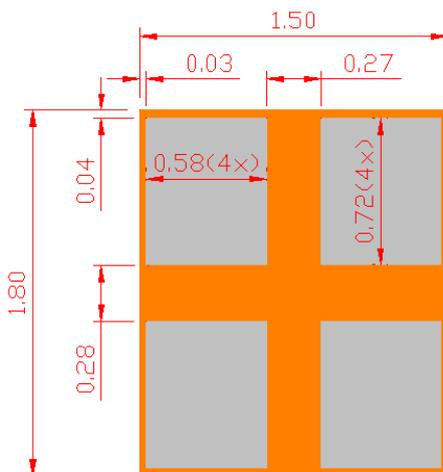
Figure 6: Paste mask detail for each pad
